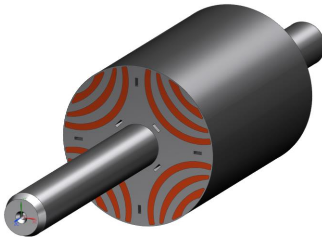
Figure 1 – Hybrid reluctance magnet
